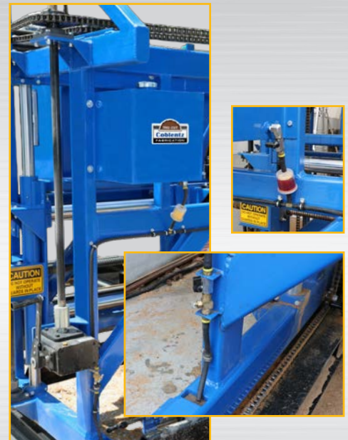
Viewing Hydraulic Cutterhead Motor, Rubber Coupler, Bearing, and Cutterhead Arborshaft
