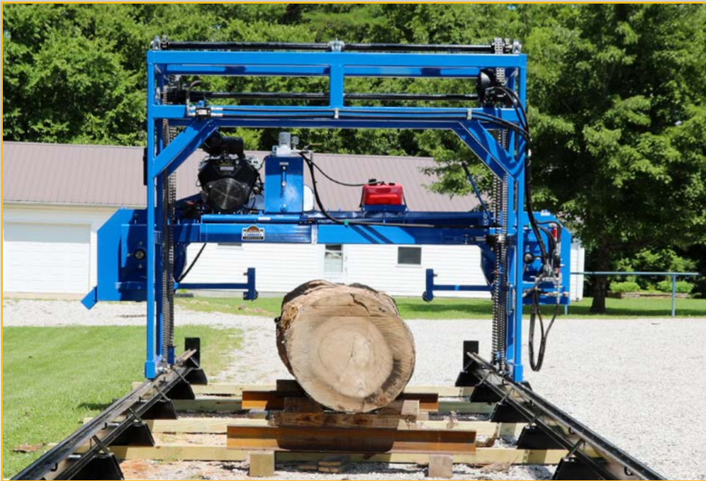
Rear view of HS-96 on concrete slab track with track riser blocks. This photo shows how concrete slab track can be set up on 6 x 6 posts in a temporary or remote location to do milling.
