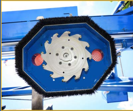
Viewing 14" diameter 12-Tooth Replaceable Carbide Cutter with adapter machined in bottom to receive sanding head.
