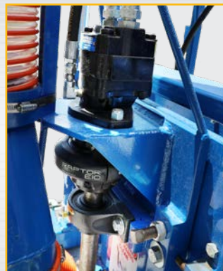
Viewing Hydraulic Cutterhead Motor, Rubber Coupler, Bearing, and Cutterhead Arborshaft
