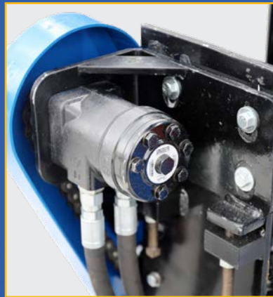
Hydraulic motor powers a 20-1 Gear Reducer for powerlift of Cutterhead.
