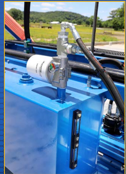
Viewing 90 Gallon Hydraulic Oil Reservoir with Return Filter and Oil Level Temperature Gauge
