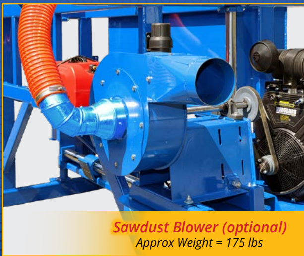
Blower Belt Guard removed to show clarity
